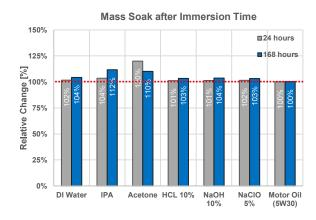
ASTM D543: Samples immersed in different chemicals were stored at 22°C. Samples immersed in Motor Oil were stored at 50°C. Properties of media used: pH(HCl, 10%) = 1; pH(NaOH, 10%) = 14; pH(NaClO, 5%) = 13
